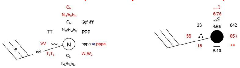
Decode of elements plotted on a land station circle (note the colour coding)
